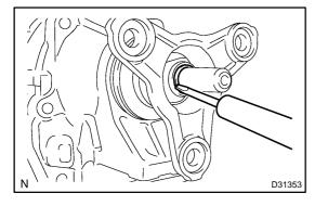
Remove the nut and flange yoke assy. (b)
