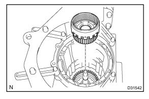
Install the front planetary ring gear and the thrust needle (a) roller bearing to the case.
