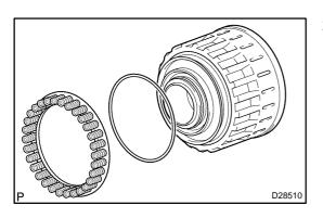
Check whether the sliding surface of the disc, the plate (a) and the flange are worn or burnt. If necessary, replace them.
