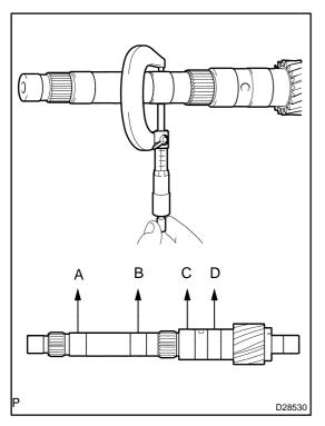
(b) Using a micrometer, check the outer diameter of the intermediate shaft positions shown in the diagram.
