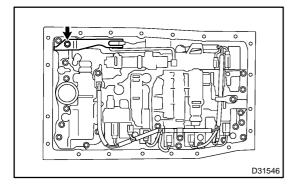
(c) Install the detente spring with the bolt.
