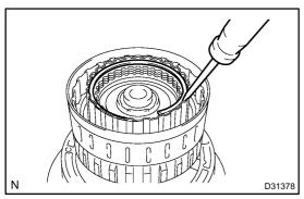
12. REMOVE FORWARD MULTIPLE DISC CLUTCH CLUTCH DISC
