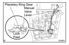
Shift the manual valve lever to the P position, and confirm (b) the planetary ring gear is correctly locked up by the lock pawl.
