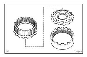
(b) Remove the CTR planetary ring gear and the front planetary ring gear flange from the front planetary ring gear.
