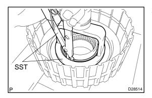
28. REMOVE DIRECT CLUTCH PISTON SUB-ASSY
