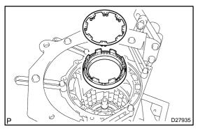
50. REMOVE BRAKE PISTON RETURN SPRING SUB-ASSY
