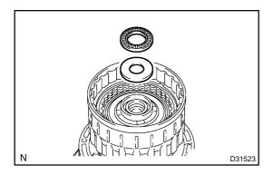
(c) Remove the thrust needle roller bearing and thrust bearing race from the clutch drum assy.
