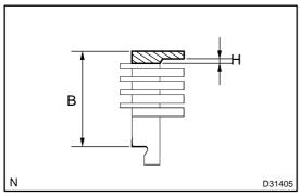
(c) Using vernier calipers, measure the thickness (length B) of the brake flanges the 4 brake plates No.4 and the 4 brake discs No.4 altogether at the both ends across a diameter, and calculate the average.
