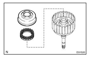
(c) Remove the clutch balancer No.1 and the forward clutch return spring from the input shaft assy.
