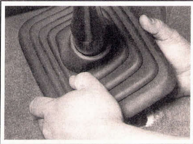
2.4 Remove the retaining screws, then slide the boot and the boot insulator off the shift lever
