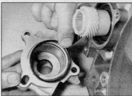
6.7b . . . and remove the housing, sealing ring and drive pinion from the transmission
